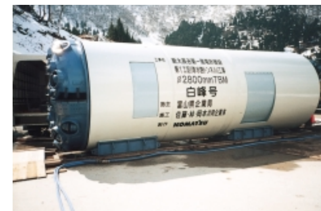
Excavation and covering integrated TBM
