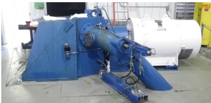
Photo-1 250kW Turgo impulse turbine and generator
